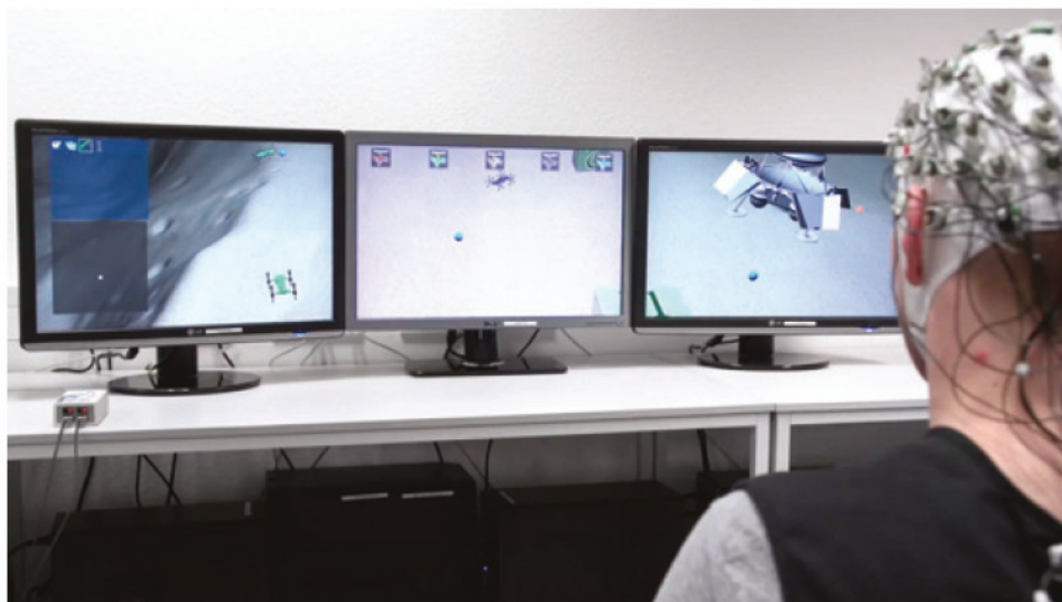
Figure 14.13 Video: Virtual multi-robot control in 2D using a multi-PC system supported by embedded brain reading. https://www.youtube.com/watch?v=zeFp_JBSBxA
