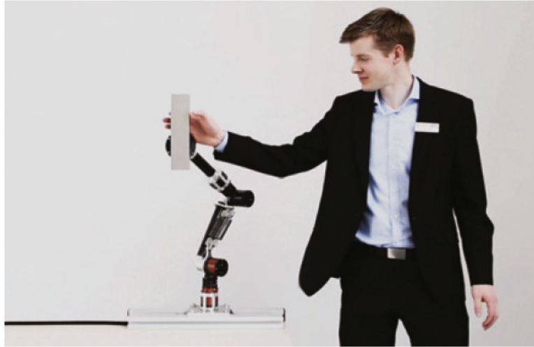
Figure 14.2 Video: The COMPI arm: compliant trajectory tracking via model-based control allows safe human-robot interaction. https://youtu.be/mDODMNM5zc .
