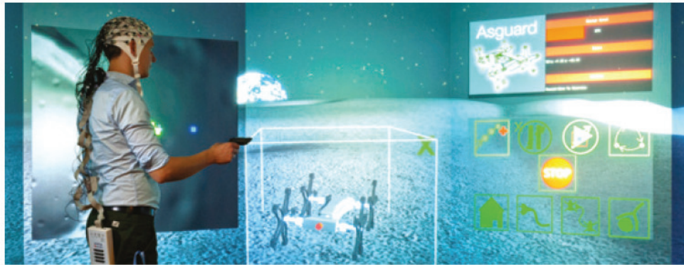
Figure 14.12 Immersive virtual 3D multi-robot control using a CAVE. Figure courtesy of [Kirchner and Drechsler 2013].
