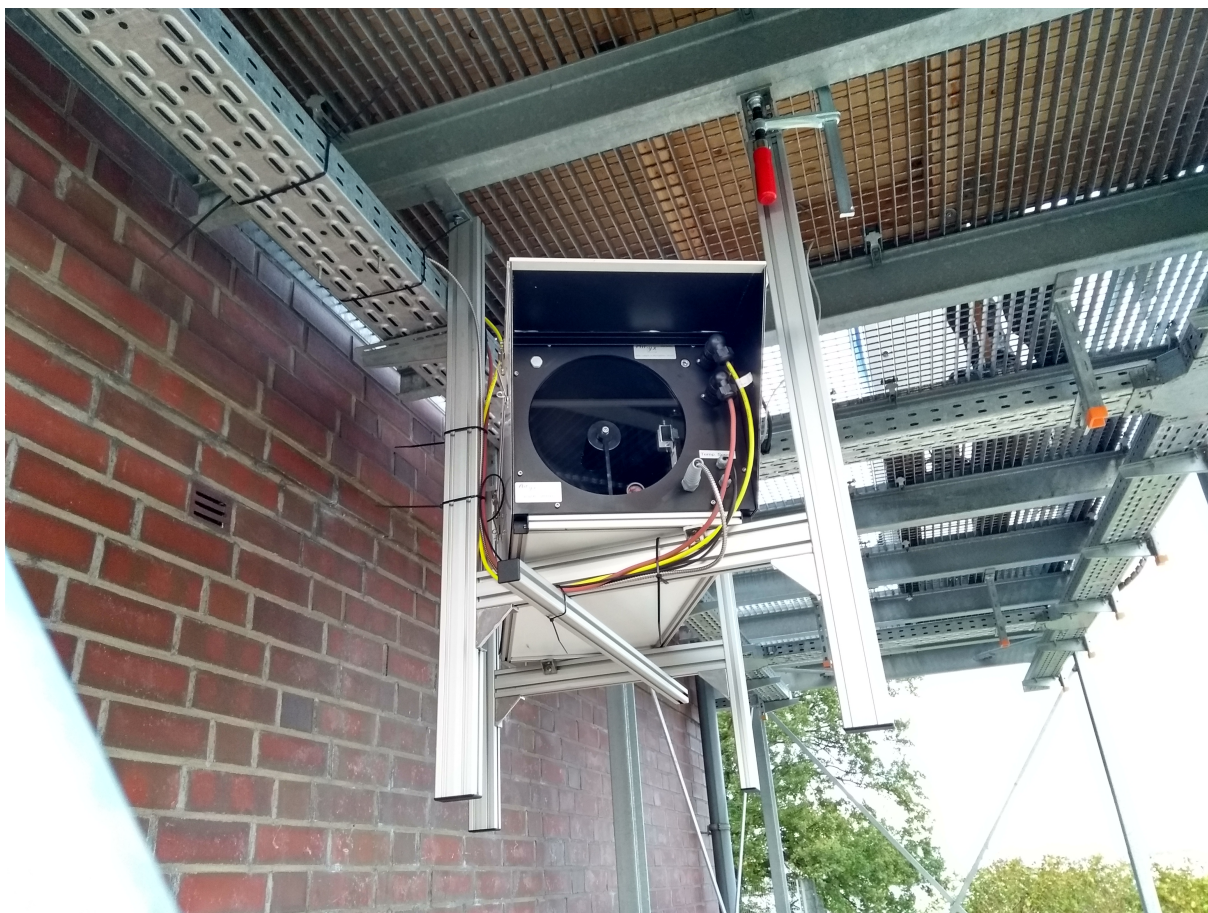
Figure 5.1: Telescope unit of the Airyx LP-DOAS instrument.
