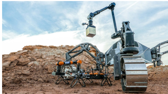
Figure 2: Multi-Robot Scenario: SherpaTT is handing over a sample container to CoyoteIII for return to the lander. CoyoteIII has the modular manipulation arm SIMA attached which is currently in a pose to facilitate the container hand-over.
