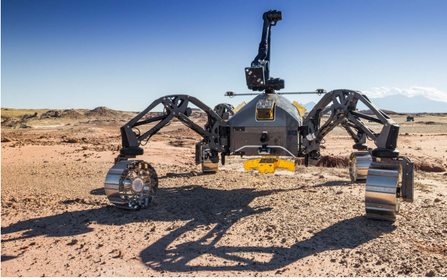
Figure 1: The hybrid wheeled-leg rover SherpaTT during the field test campaign. In the photograph, the system is equipped with modular units used in a multi-robot scenario. The two antennae of the DGPS-system used for ground truth-data can be seen behind the central manipulator.
