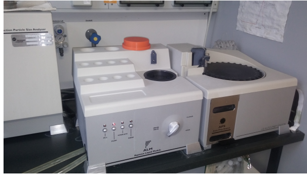
Figure 2.8: Beckman Coulter Laser LS 13320 at MARUM laboratories for grain size measurements.
