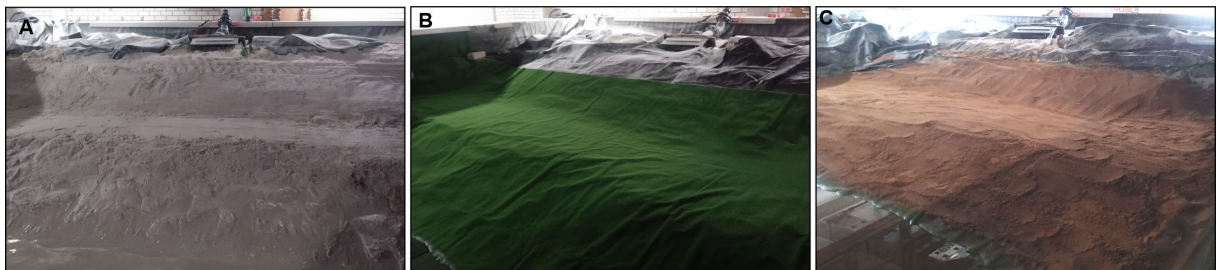
Figure 2.9: Photos showing the setup of the experimental site in the flume tank. (A) Morphology built with sediment. (B) Morphology covered with artificial grass. (C) A thin layer of crushed walnut shell on top of artificial grass.
