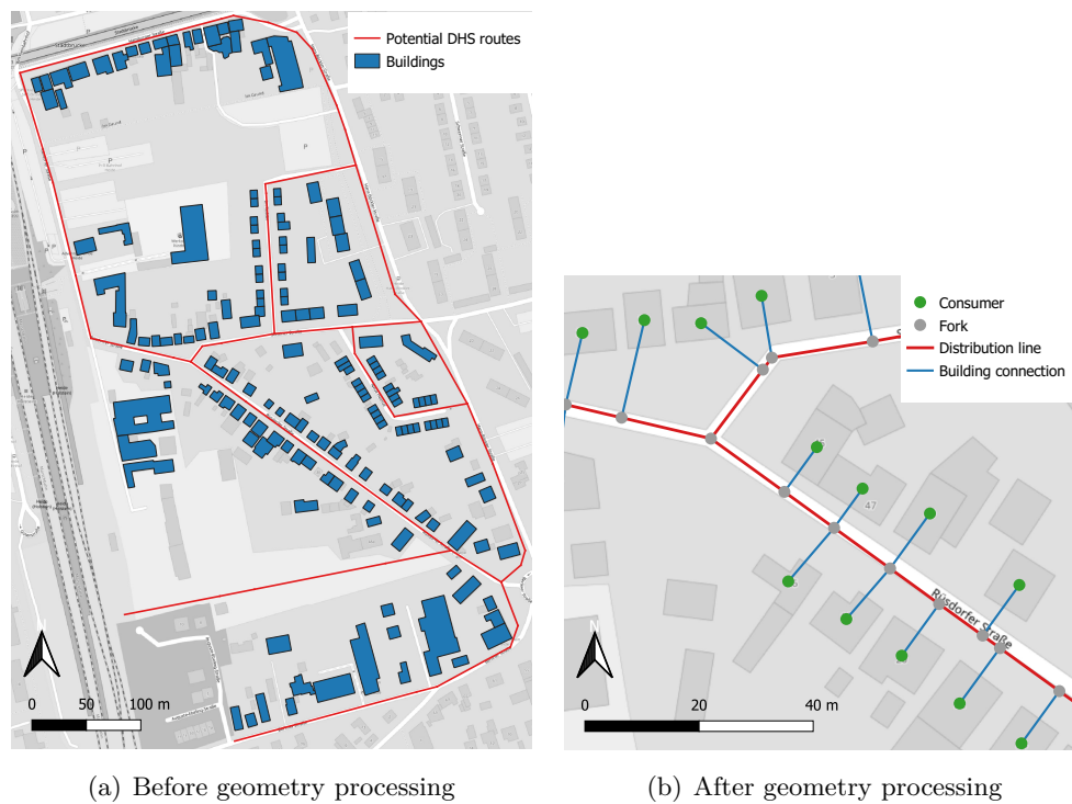
Figure 3.1: (a) Geometry input of the district planning and optimization approach. Red: possible district heating routes; blue: considered buildings. (b) Result of the geometry processing and input for the optimization model. Source background map: (OpenStreetMap contributors 2022).
