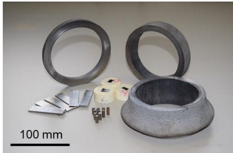
Figure 1-1: Samples from spray-formed steel tube produced by a close-coupled atomizer.
