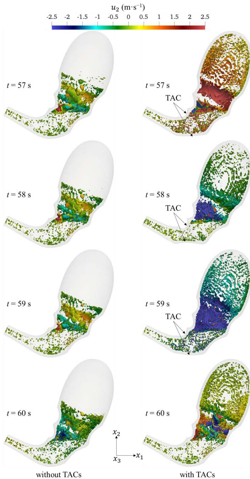
Fig. 5.8. Vortical structures identified with Q = 0.001 \text{ s}^{-1} , colored with the vertical velocity component u_2 .
