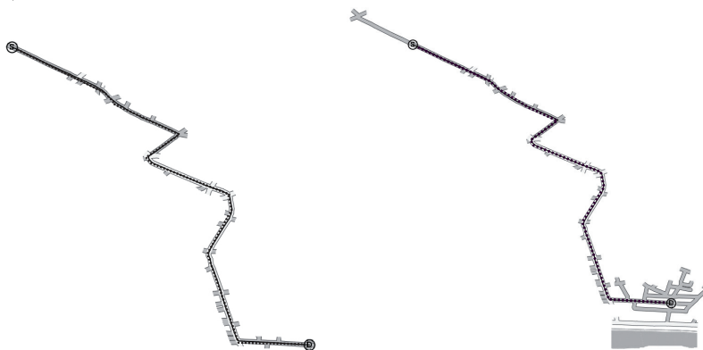
Figure 9: a) shows the original (survey) map with the route (thin black line) from S to D. b) shows the extracted route, c) the route with disambiguated start environment and extended destination environment.
