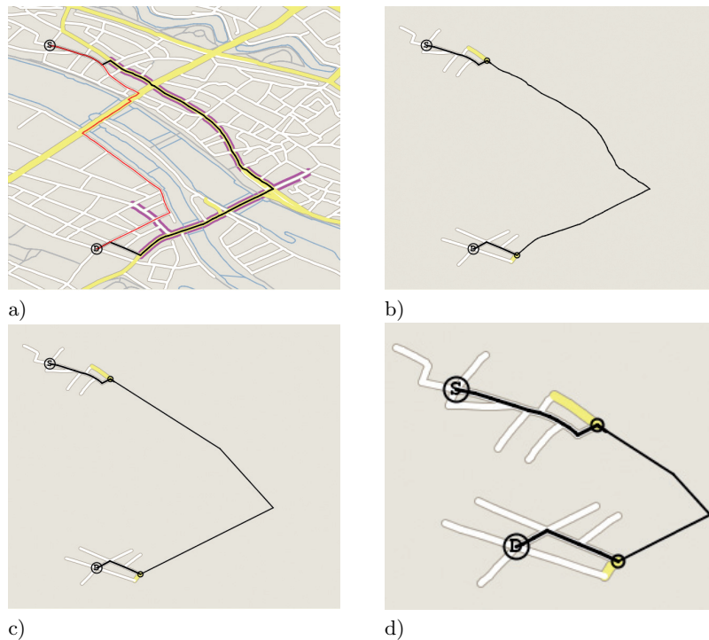
Fig. 1. Generating a \mu Map: The map in a) shows the map annotated with previous knowledge (bold magenta/dark gray lines), the shortest path from S to D (red/light gray), and the path across prior knowledge (black). In b) we see the unfamiliar segments of the route connected by the path across previous knowledge. In c) the prior knowledge path is schematized. In d) the familiar, schematized path is minimized by means of the convex hull distance, and the unfamiliar segments of the route are moved towards each other. The final \mu Map in d) is significantly smaller than the original map in a).
