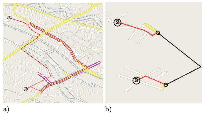
Fig. 1. Generating a \mu Map: a) depicts the original map annotated with prior knowledge (bold magenta lines), the shortest path from S to D, and the path across previous knowledge. b) shows the corresponding \mu Map: the path across the prior knowledge is schematized and minimized, the unfamiliar parts are visualized in detail. Note the different space requirements of a) and b).
