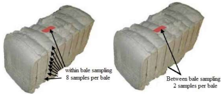
Fig. 4.2 Within-bale (left) and between bale (right) variability sampling. (Gourlot J.-P. and Drieling A., ISBN: 978-2-87614-686-0. EAN: 9782876146860 [62])
