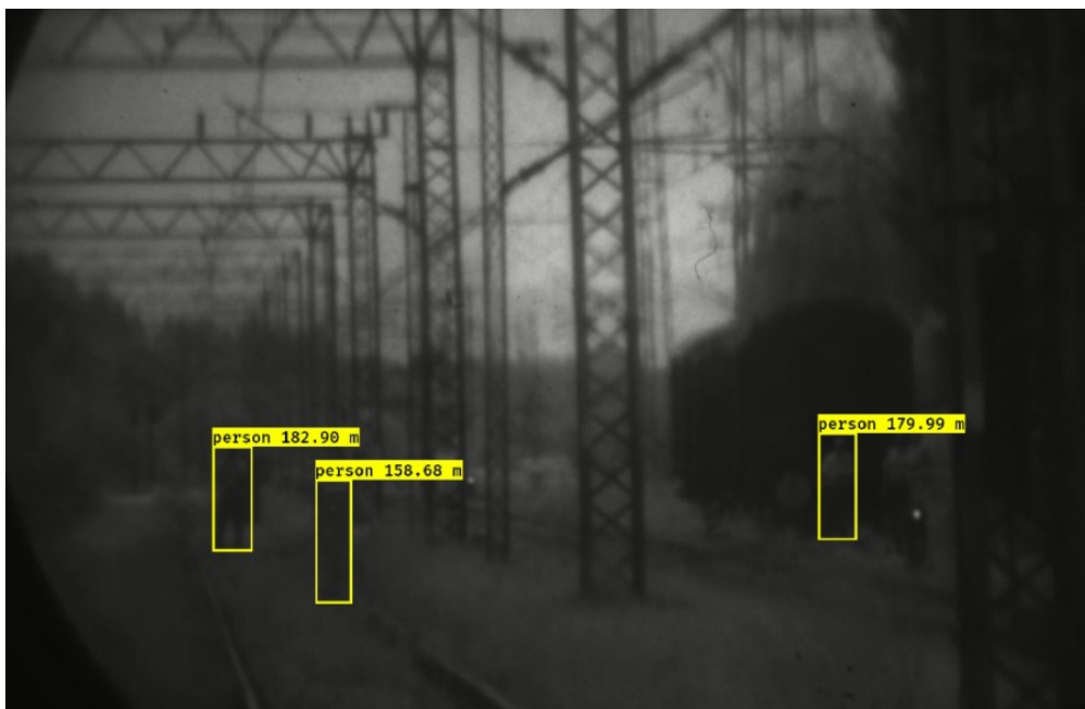
Figure 66. Object detection and distance estimation in onboard thermal camera image recorded in the environmental condition of 38°C; Good detection result in spite of low-contrast image; Ground truth distance for a person: 155 m (0.025 %)
