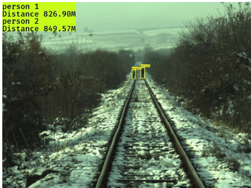
Figure 58. Object detection and distance estimation in RGB camera image recorded in winter (snow) environmental conditions; Ground truth distance: 835 m (0,97 % and 1,74% respectively).
