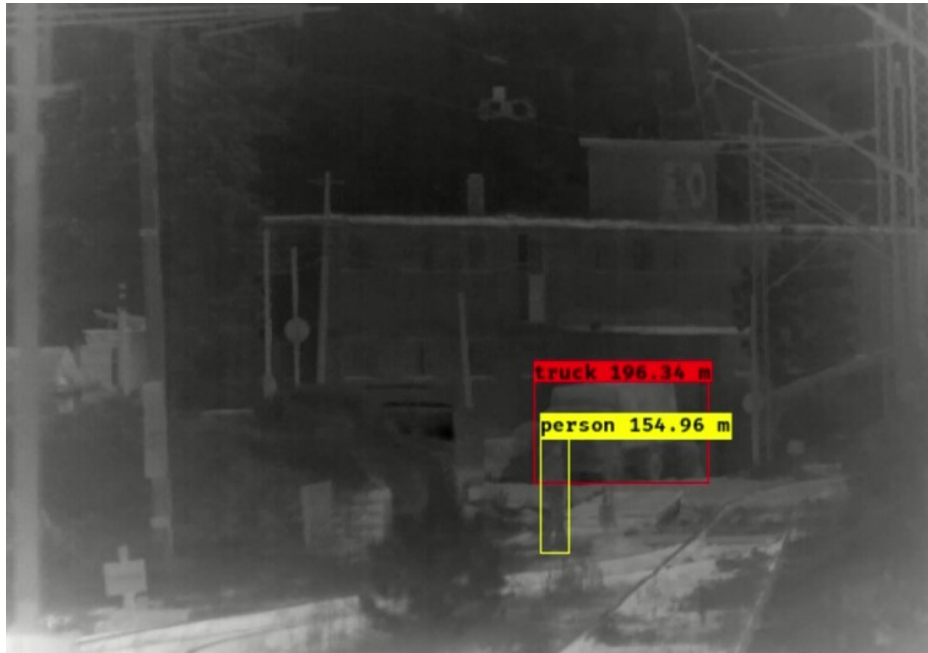
Figure 66. Object detection and distance estimation in onboard thermal camera image recorded in the environmental condition of 38°C; Good detection result in spite of low-contrast image; Ground truth distance for a person: 155 m (0.025 %)
