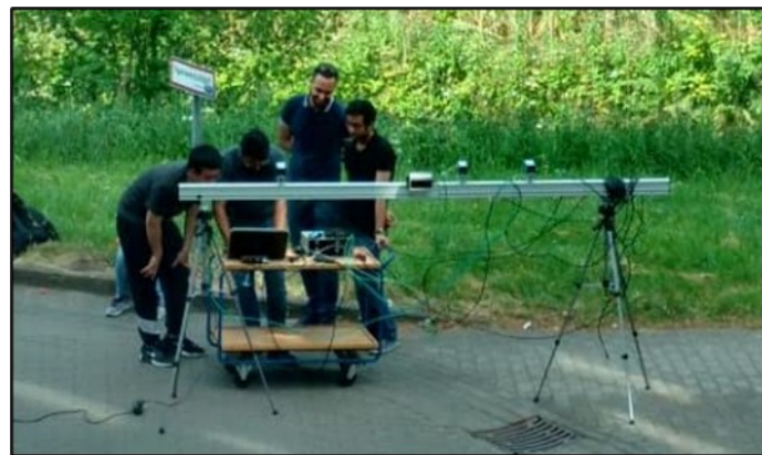
Figure 37. Field tests performed in University Campus. Test-stand with the vision sensors and laser scanner.
