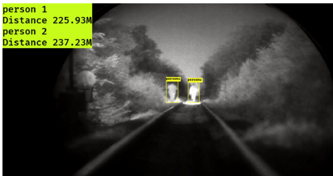
Figure 61. DisNet estimation of distances to objects in a rail track scene from the night vision images.
