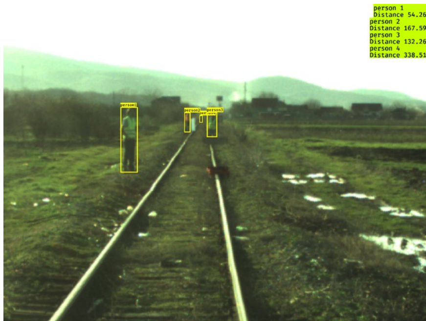
Figure 57. DisNet estimation of distances to objects in a rail track scene from the RGB camera image. Magnified RGB image overlaid with bounding boxes and distance estimation of detected persons at 50, 100, 150, and 300 m respectively.
