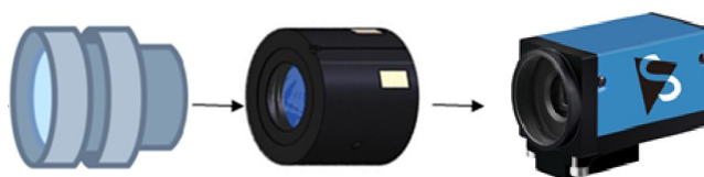
Figure 34. A monochrome CMOS camera sensor equipped with image intensifier and objective lens [116]
