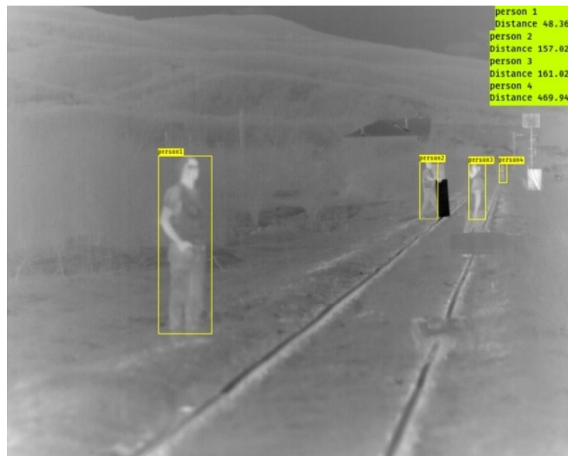
Figure 60. DisNet estimation of distances to objects in a rail track scene from the thermal images. Distance estimation of detected persons at 50, 100, 150 and 500 m respectively
