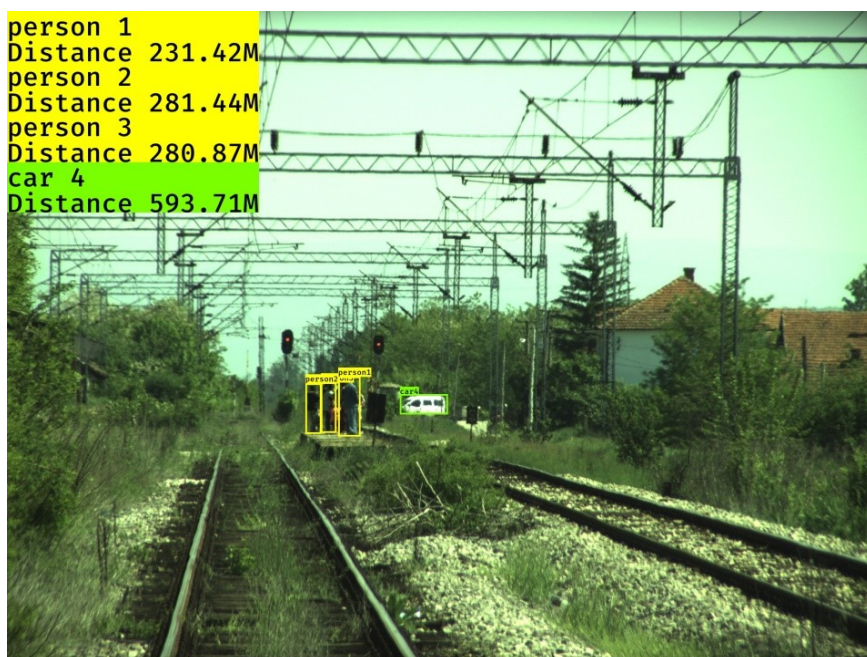
Figure 65. Mid- to Long-range object detection and distance estimation in on-board RGB camera (zoom) image; Ground truth distance: for persons (station middle point) 266.69 m (average error 8.32%), for the car 597.87 m (error 0,69%)
