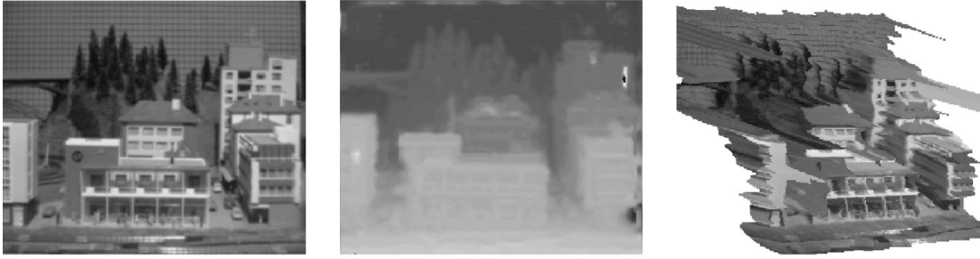
Figure 28. Input – First frame (left image), Depth image (center), Prespective view (right) [100]
