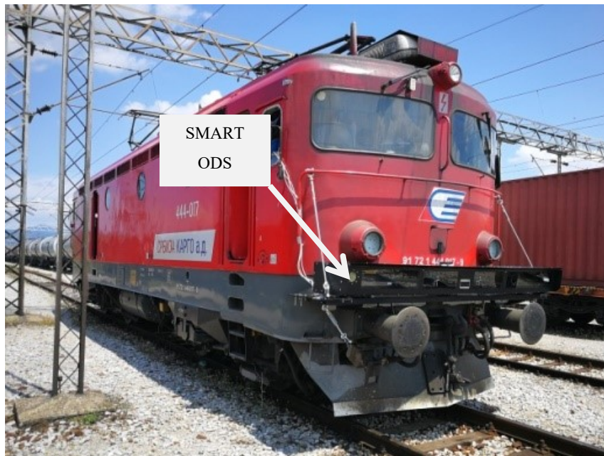
Figure 94. Vision sensors for obstacle detection integrated into sensors' housing mounted on the frontal profile of a locomotive below the headlights [120]
