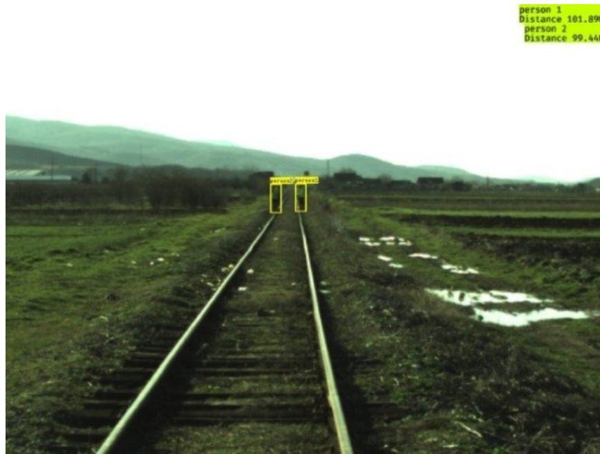
Figure 56. DisNet estimation of distances to objects in a rail track scene from the RGB camera image. Distance estimation of detected persons at 100 m
