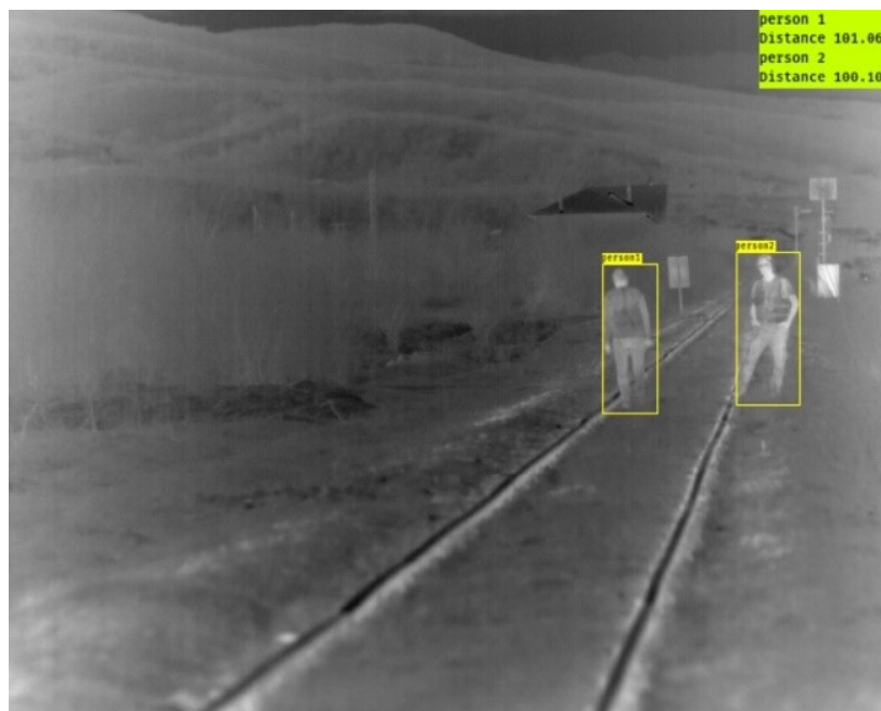
Figure 59. DisNet estimation of distances to objects in a rail track scene from the thermal images. Distance estimation of detected persons at 100 m
