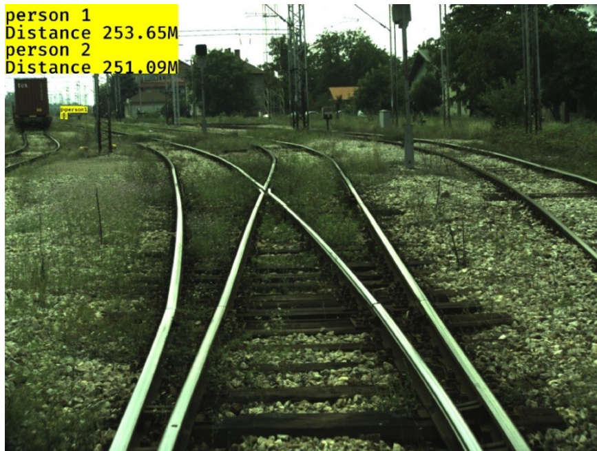
Figure 64. Mid-range object detection and distance estimation in on-board RGB camera image; Ground truth distance: 231.97 m (errors 8.2% and 8.24% respectively)
