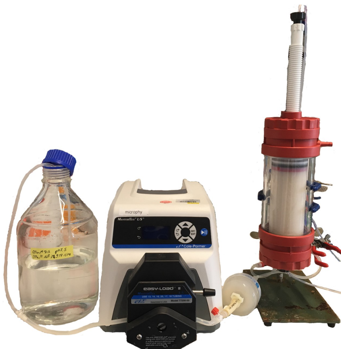
Supplement Figure 1: A simple medium-scale setup for the purification of fucoidans. The peristaltic pump was manually controlled to load, wash or elute fucoidans onto the column packed with ANX-FF resin. The duration of one run, including column wash was approximately 45 minutes and yielded up to 350 mg of purified fucoidans per 500 mg starting material.
