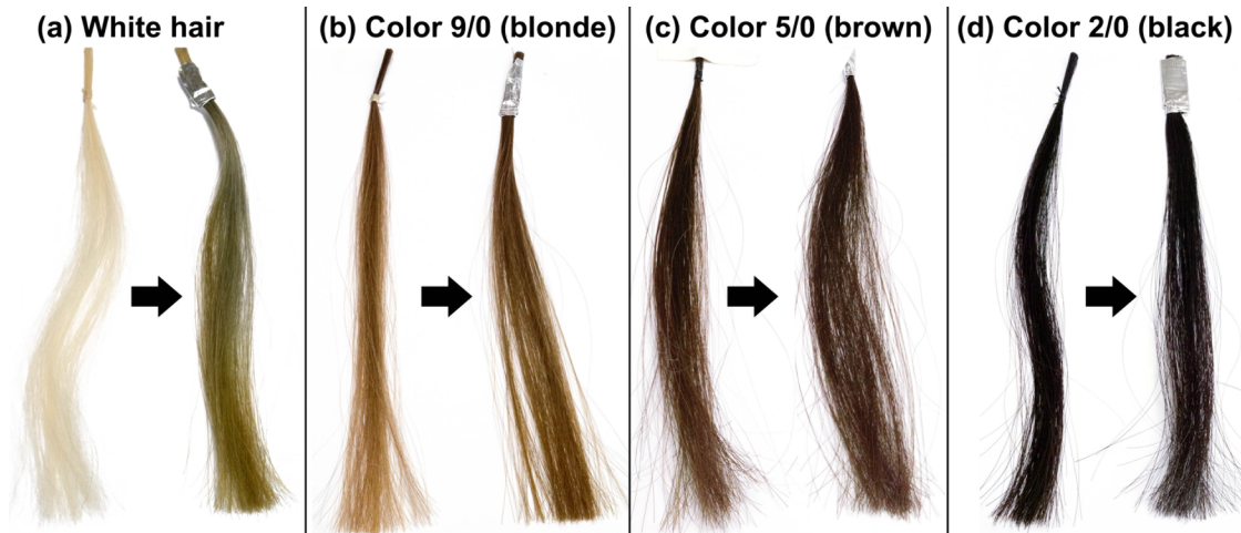
Figure 59 - Images of four different hair colors in their virgin and treated state. (a-d) On the left the virgin sample and followed by an arrow, the coloring effect. The length of free hair is 13 cm and each sample weights 0.4g (+/- 0.05g of tolerance). The color codes were provided by the supplier of these samples (Kerling International).
