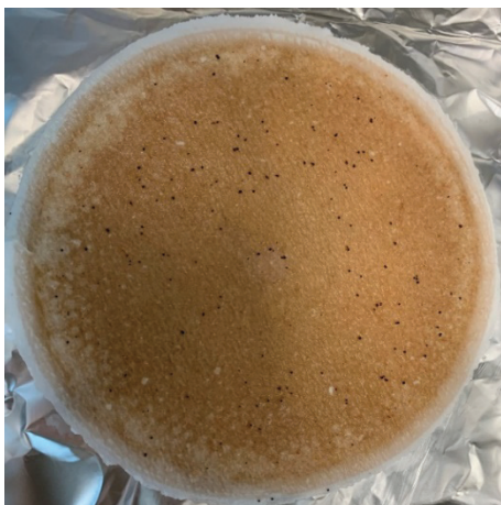
Fig 3.3: POC filter with plenty of particulate material. 50 L of seawater from the ship inlet were filtered using a peristaltic pump through 0.47 \mu\text{m} GF/F filters with a diameter of 142 mm.
