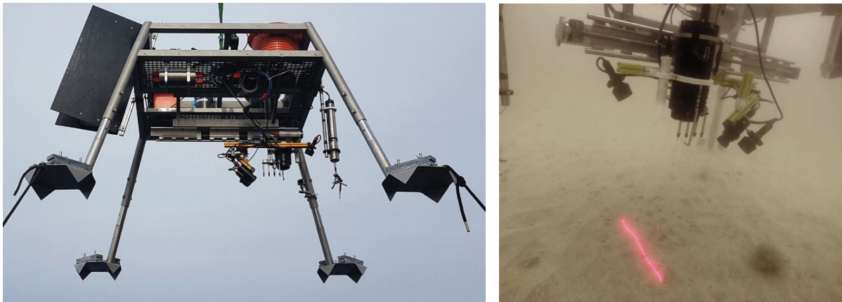
Fig. 3.10: Left panel: LanceALot after a 24 hour deployment on the Mauretanian shelf. Right panel: Surface-scan of the sea-floor using a laser-scanning technique.
