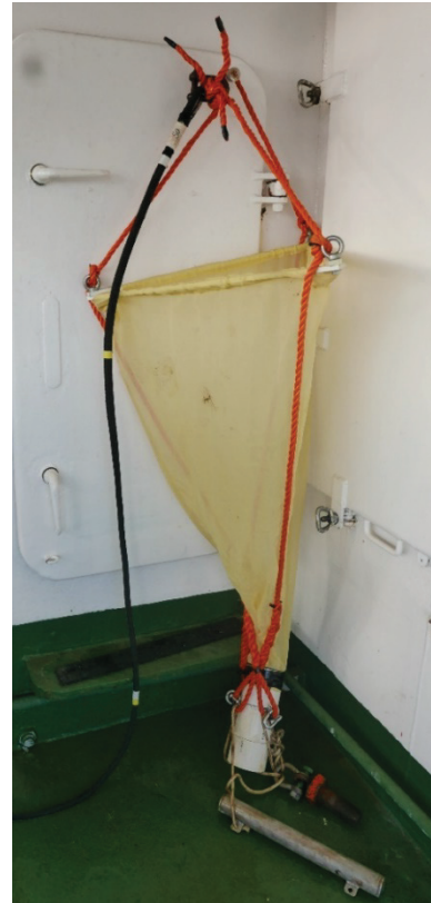
Fig. 3.2: Zooplankton hand net with weight attached.
