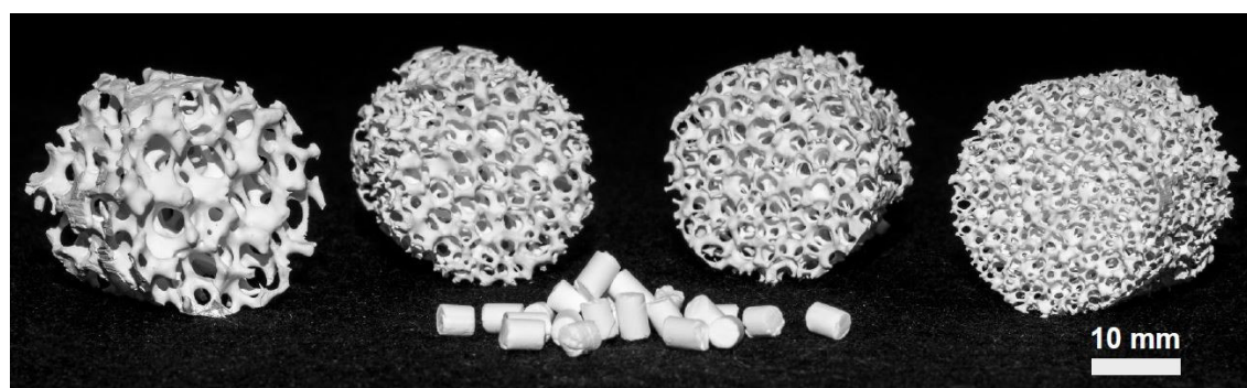
Figure 2.13 Examples of catalyst supports in heterogeneous catalysis. Background: solid mullite sponges with decreasing pore window size from left to right. Foreground: alumina pellets [157].
