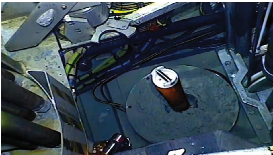
Fig. 5.24 Picture showing the observatory sealing the drill string that is reaching 20 m into the summit of Ginsburg MV shortly before the MeBo is lifted from the seafloor.
