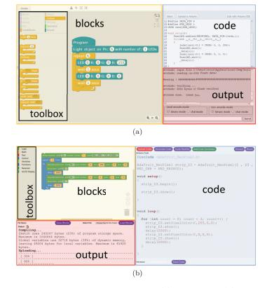
Figure 6.1: A view of the user interface for the (a) mBlock and (b) micro-controller part of BEESM (MpB).
