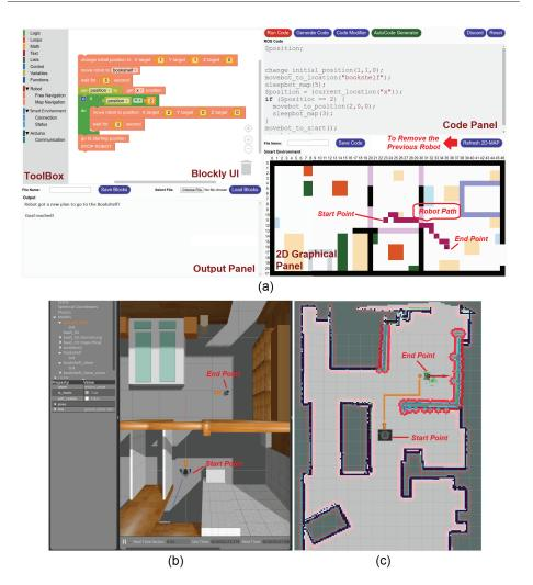
Figure 3.3: An overview of (a) BEESM user interface together with (b) GAZEBO robot simulation, and (c) RViz for ROS.
