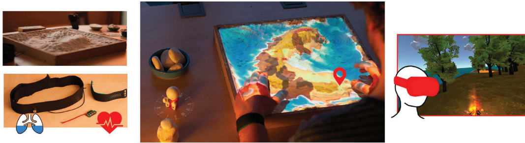
Figure 2.2: InnerGarden system for mindful practices. User’s heart rate and breathing is reflected in VR, mirroring bodily state for self-reflection. Image source: Roo et al. (2017).
