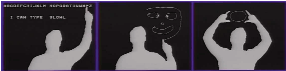
Figure 2.8: Videoplace system by Krueger et al. (1985) demonstrating natural gesture interaction: typing, drawing, and pinching. Source: Myron Krueger (1985).
