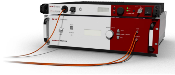
Fig. 3.7: High power laser system NKT Koheras BOOSTIK consisting of a narrow linewidth laser on top of an amplifier with an output power of 10-15 W (image by NKT Photonics [172]).
