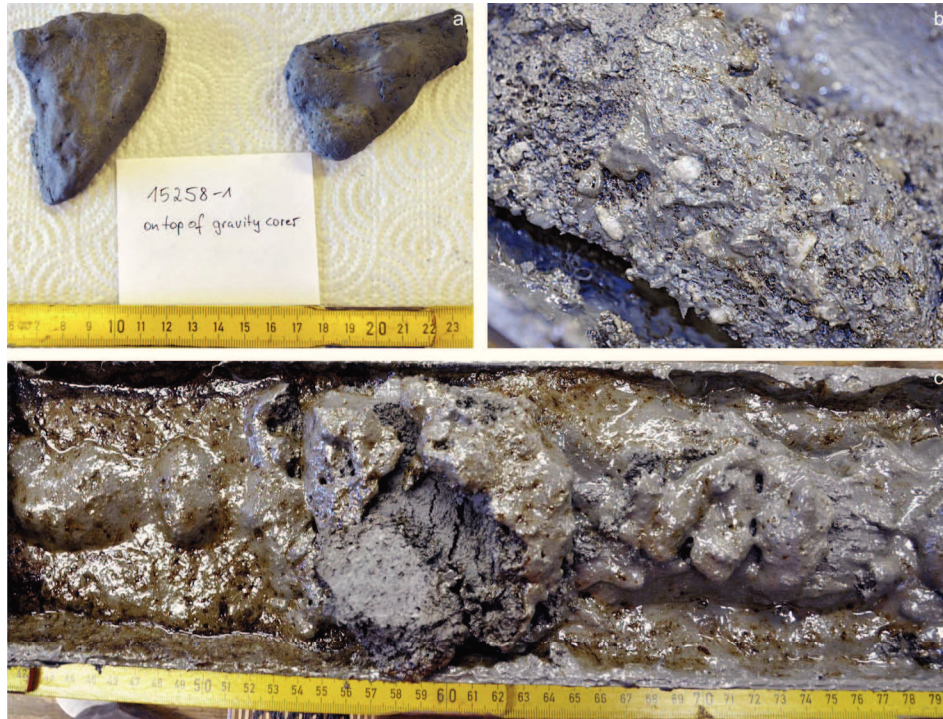
Fig. 57. Photographs of sediment samples from oil seep G2 at Kulevi Ridge (see Fig. 51 for location). a) Two mud clasts recovered on top of the gravity core. b) Millimeter-sized gas hydrate grains were dispersed throughout the core. c) Oil stained, muddy sediments of upper half of the core.
