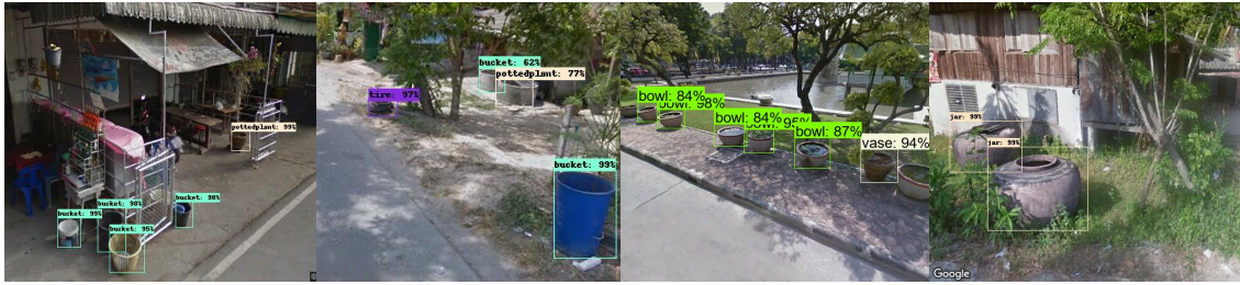
Figure 5. Examples of detected containers in Google street view images by using Faster R-CNN with new transferred categories. Original images © 2018 Google, Chatuchak, Bangkok
