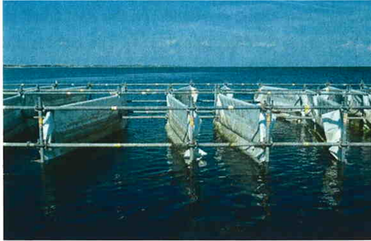
Fig. 2. Three-current-flume. Close-up view of three flume lanes with different openings thus manipulating current velocity into increased, unaltered or reduced flow across the mid section of the flume. Measurements: 8 m length, 12 m width, 1 m height. Photo: Anja Schanz
