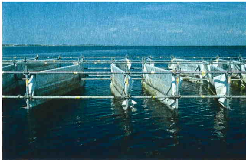
Fig. 2. Three-current-flume. Close-up view of three flume lanes with different openings thus manipulating current velocity into increased, unaltered or reduced flow across the mid section of the flume. Photo: Anja Schanz
