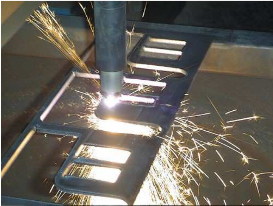
Figure 1.1: Plasma cutting process
