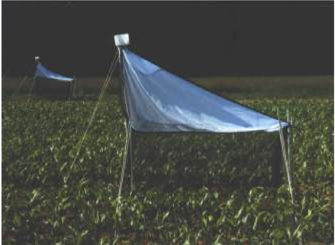
Figure 7: Malaise trap for recording flying insects to assess the potential prey spectrum for orb-web spiders.
