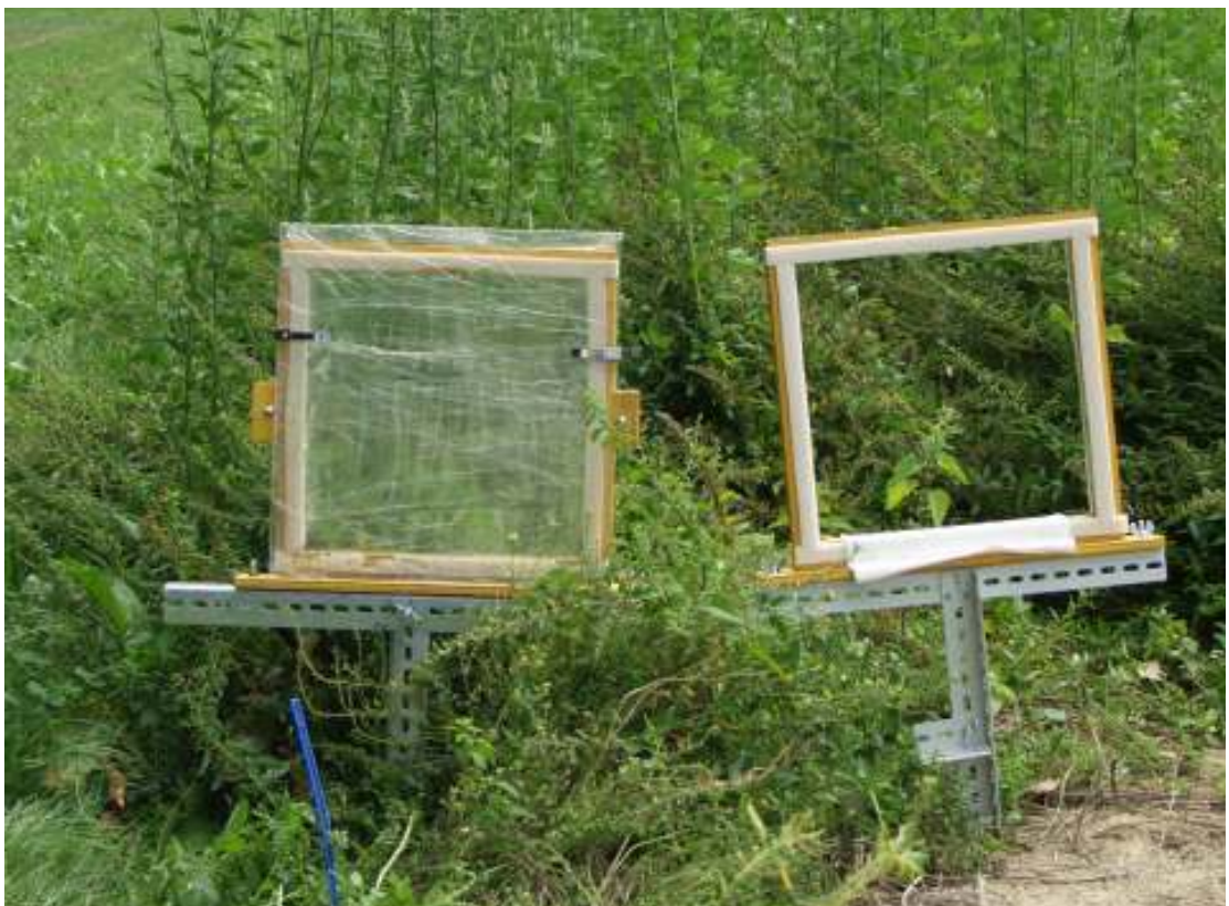
Figure 8: Sticky trap consisting of plastic plates covered with a clear film spread with non-drying sticky glue (left) for recording the potential prey spectrum beside a orb-web spider and its web built in a wooden frame (right) for recording the actual prey spectrum of the orb-web spider.
