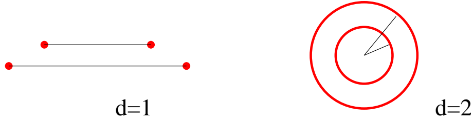
Figure 4.5. Geometry of coarse coding. For each tuning function the area of positive Fisher information corresponds to the surface of a d -dimensional sphere with radius w , which is proportional to w^{d-1} .
