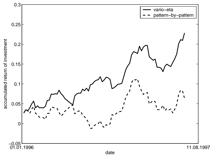
Figure 5.12 Comparison of resulting accumulated model returns using (i.) vario-eta and (ii.) pattern-by-pattern learning for the network training. The accumulated return is measured on the generalization set.
