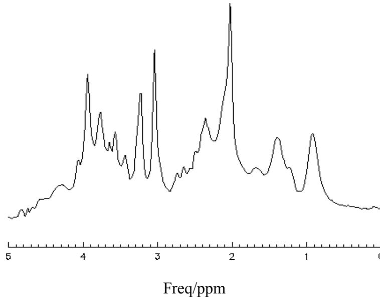
**Fig.3.3-2** *In vivo* spectrum of rat brain measured with the same pulse sequence as in Fig.3.3-1. Water residues around 4.7 ppm were removed by the Matrix Pencil based method. Only zero order phase correction was performed in time domain automatically.
