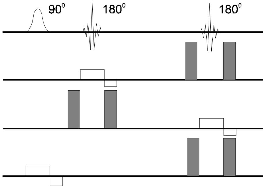
**Fig.1.3-2** PRESS sequence. The gradients in shade are spoilers and the in solid lines are the slice selective and the refocusing gradients.
