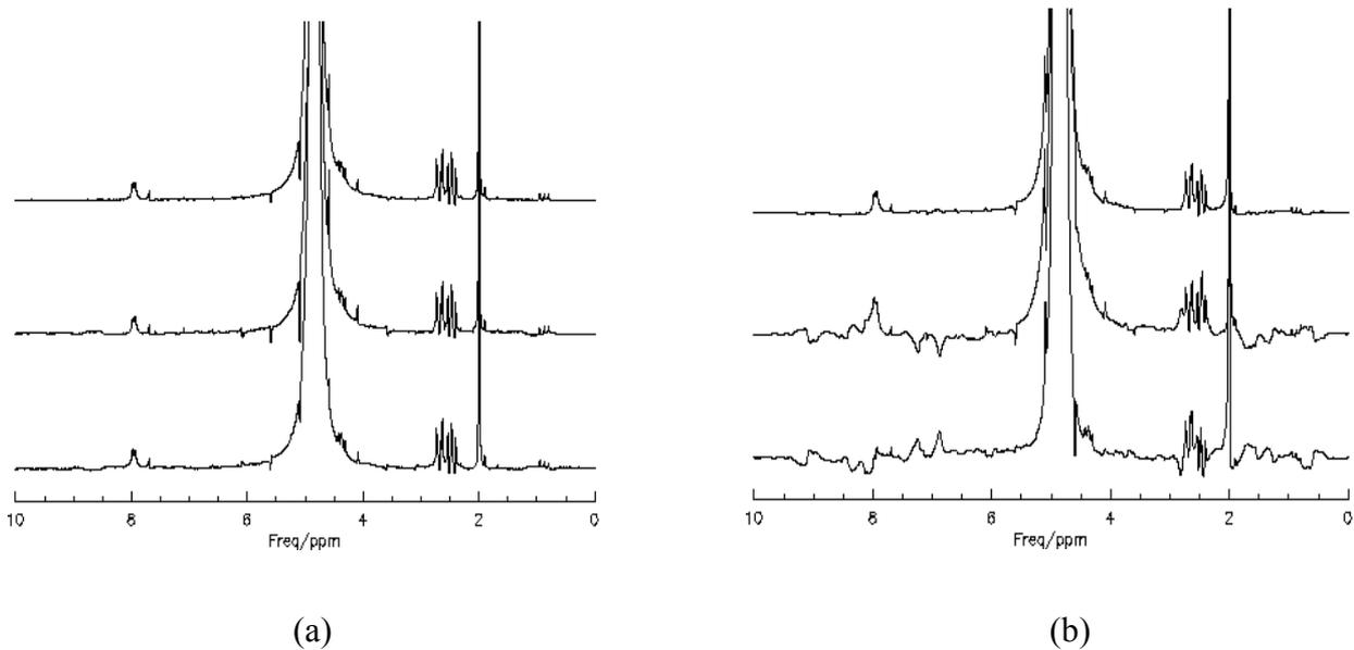
**Fig. 3.4-10** Water unsuppressed spectra of the NAA solution (100 mM) measured without spoilers (a) and with spoilers (67 mT/m). In both a and b, spectra from bottom to top are: with positive gradient pulses, with negative gradient pulses and the combination of the two.
