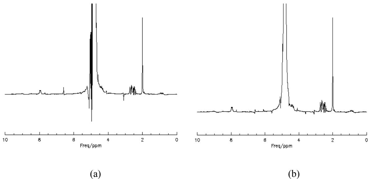
**Fig.3.4-8** Water unsuppressed proton MRS of a NAA phantom measured without spoiler gradient pulses and without phase cycling (a), and with a 16-step phase cycling (b).
