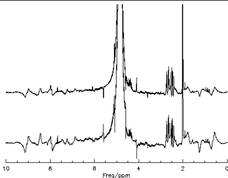
**Fig.3.4-6** Water unsuppressed spectra with spoiler gradient strengths of 67 mT/m (lower trace) and 34 mT/m (upper trace). The refocusing gradient pulses were trimmed separately for each spoiler strength. A 16-step phase cycling was used to eliminate the remaining unwanted signals in the case of smaller gradient pulse strength. Other parameters were the same.
