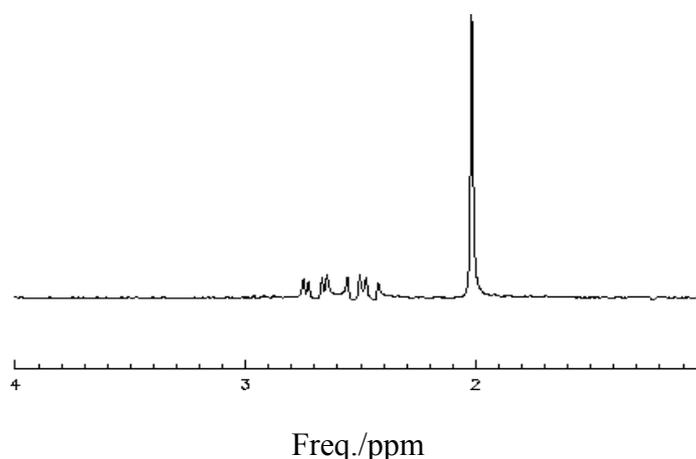
**Fig.3.3-1** NAA spectrum measured with optimally timed pulse sequence (PRESS), TE = 20 ms, with water suppression. Zero order phase correction was performed in time domain. No post-acquisition first order phase correction was performed.
