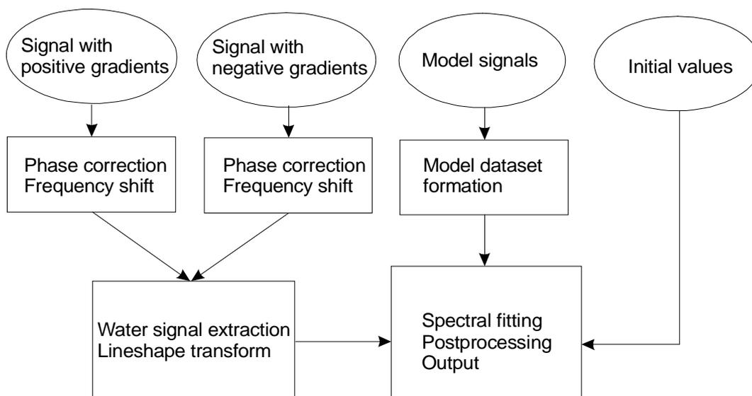
**Fig.3.7-1** Flowchart of data preprocessing and spectral fitting.
