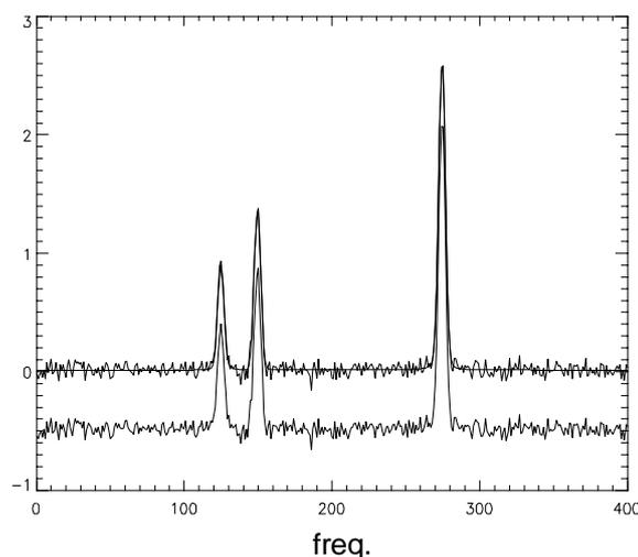
**Fig.3.7-2** An example of spectral fitting in the MC study. The lower trace is the test spectrum and the upper trace are the test spectrum and the fitted spectrum overlaid. Note that the frequency axis was scaled by a factor of 0.5.
