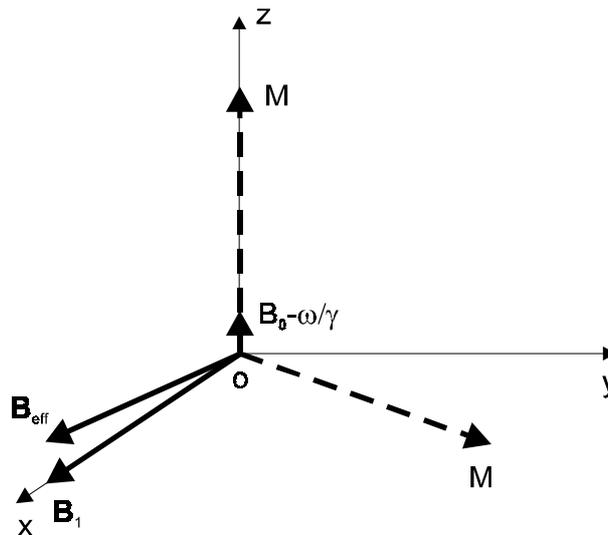
**Fig.1.1-1** Effects of total magnetic field  $\mathbf{B}_{\text{eff}}$  in the presence of RF field  $\mathbf{B}_1$ .
