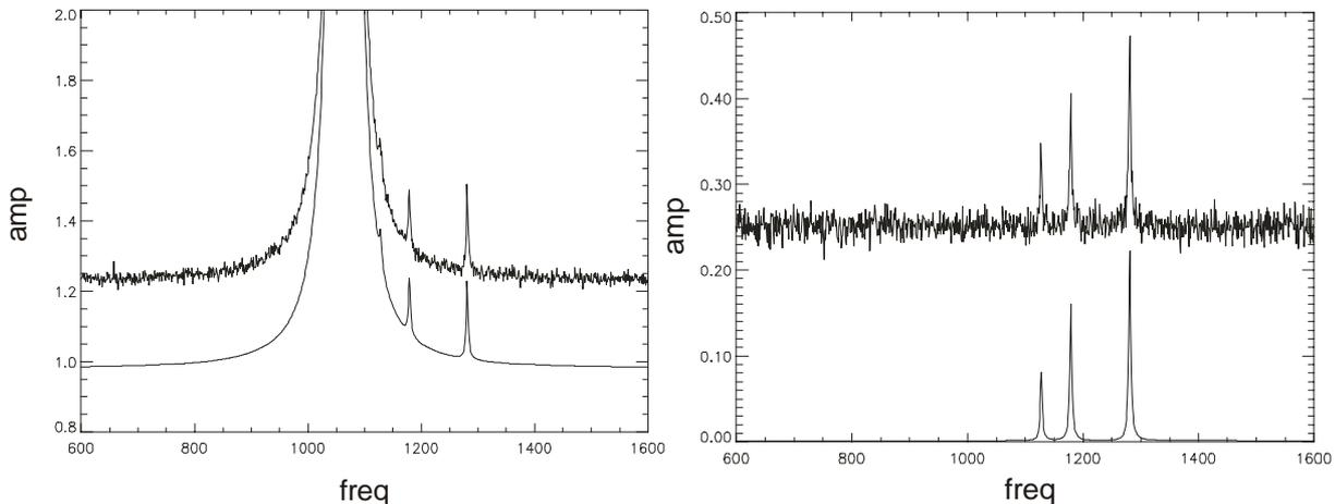
**Fig. 3.2-4** Typical spectra of synthesized and fitted signals with dominant signals (left) and after removal of the dominant signals (right). The parameters of the synthesized signals are given in Tab. 3.2.1 and the noise level is 0.5 (a.u.). Please note that the frequency was shifted and the values were not scaled to Hz.
