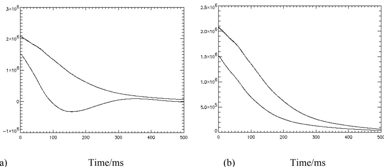
**Fig. 3.4-4** Real parts (a) of and magnitudes of FID's (b) corresponding to spectra in Fig.3.4-3. In both cases, the upper trace lines are signals measured with positive gradient pulses and the lower trace are with negative gradient pulses. Lines were broadened by 1 Hz.
