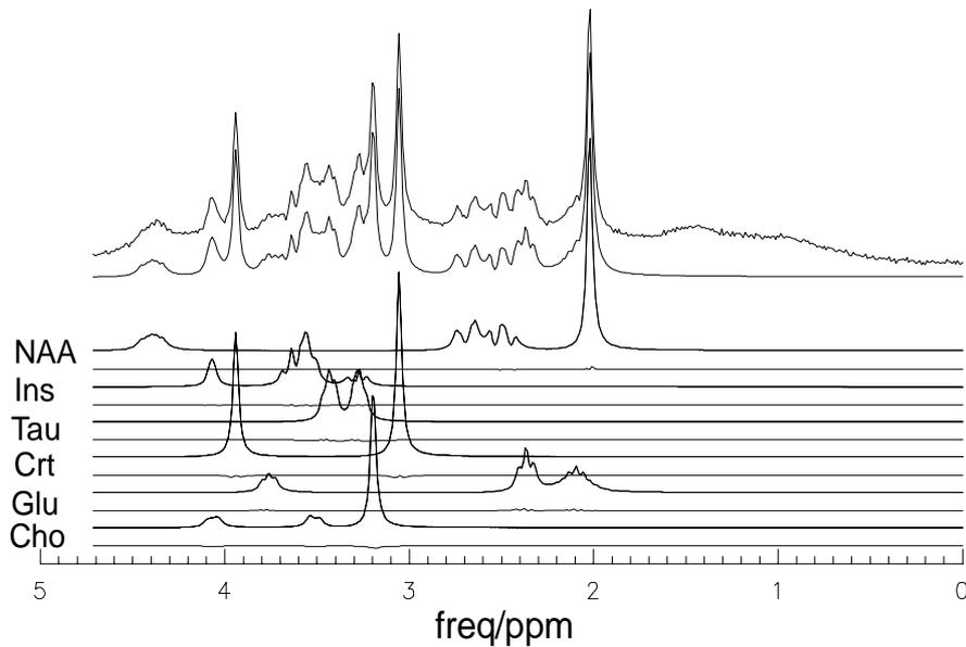
**Fig. 3.7-7** The same spectral fitting as Fig.3.7-6. From top to bottom are the total spectrum, the fitted metabolite spectrum, and the decomposition spectra of metabolites and their residues.
