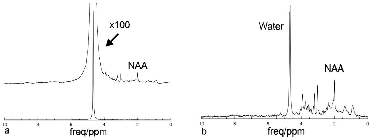
**Fig.3.1-1** Water unsuppressed (a) and water suppressed (b) *in vivo*  $^1\text{H}$  MR spectra.
