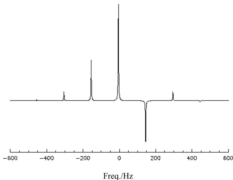
**Fig. 3.4-2** Simulated frequency modulation spectrum. A signal, called carrier signal, with zero frequency here, is frequency modulated. The modulation frequency is 150 Hz. Modulation sidebands are located symmetrically at integer multiples of modulation frequency around the carrier frequency. The pairs of odd order sidebands are anti-phase and the pair of even order sidebands are in phase.
