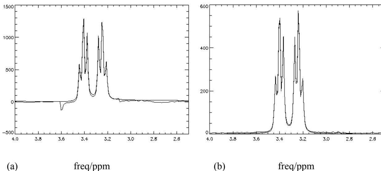
**Fig. 3.2-5** Taurine spectra measured without WS (a) and with WS (b), overlaid with the fitted spectra. The negative peak at 3.6 ppm was a frequency modulation artifact.
