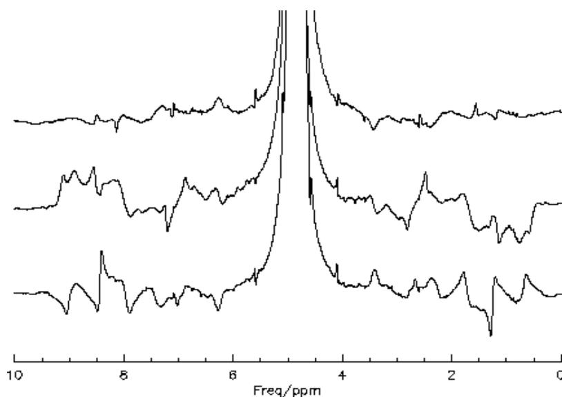
**Fig. 3.4-7** Artifacts in spectra of pure water measured with spoilers in direction x (lower trace), y direction (middle trace) and z direction (upper trace). The strength of spoiler gradients is 67 mT/m. The main magnetic field is in z direction. The interval between the spoiler gradient pulses and the acquisition time are the same in all cases.
