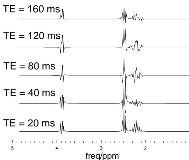
**Fig.1.2-1** Glutamate spectra at different TE's, simulated with the help of GAMMA [Smit94], a C++ library for NMR spectral simulation. Note the different patterns of the spectra at different echo times due to the J-coupling.
