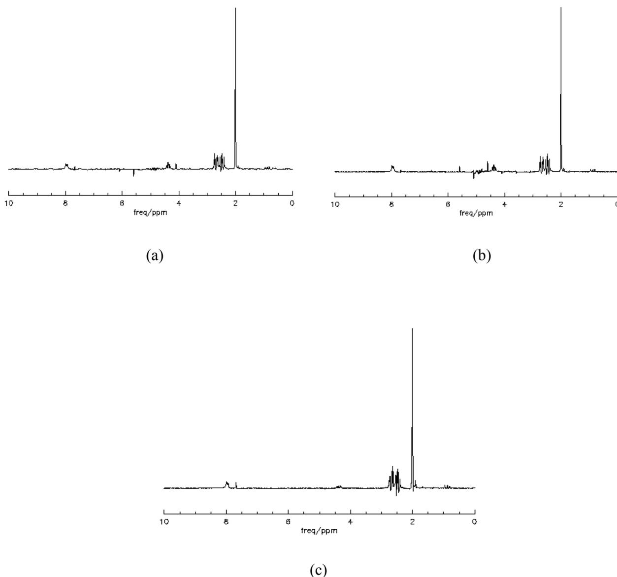
**Fig. 3.4-11** Water unsuppressed proton spectra acquired without spoiler gradients (a) and with spoiler gradients (b, spoiler = 67 mT/m), and spectrum with water suppression (c). The water signals in a and b and water residues in c were removed by Matrix Pencil Method. Water signal occurs at about 4.85 ppm. The same receiver gain was used for measurements with or without WS.
