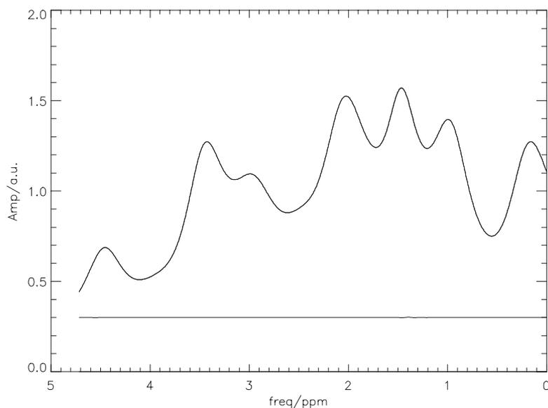
**Fig. 3.6-6** Simulated baseline overlaid with the reconstructed baseline from the wavelet coefficients of the largest 7 of total 11 scales (upper trace) and their difference (lower trace).
