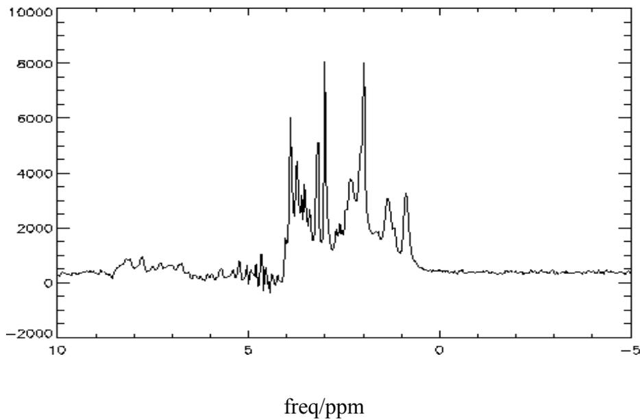
**Fig. 3.2-3** Water signal was extracted from 300 data points undersampled from original 600 points and reconstructed with 600 points. Complete water removal was reached due to perfect water signal fitting. The original data were the same as in Fig. 3.2-2
