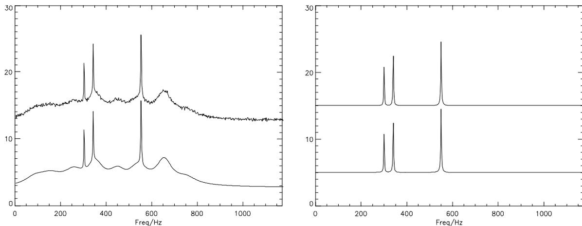
**Fig.3.7-5** A spectral fitting from the MC study: the total test (with pure spectrum, baseline and noise; left, upper) and the fitted (left, lower) spectra, and the pure spectral part of the test (right, upper) and the fitted (right, lower) spectra.
