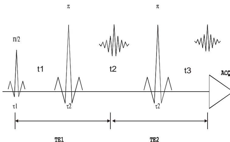
**Fig. 3.5-1** PRESS sequence used for the spectral simulation.
