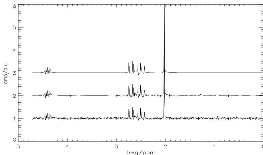
**Fig. 3.6-1** An example of wavelet denoising on simulated NAA signal. From bottom up are the noisy, the denoised and the noise-free spectra.
