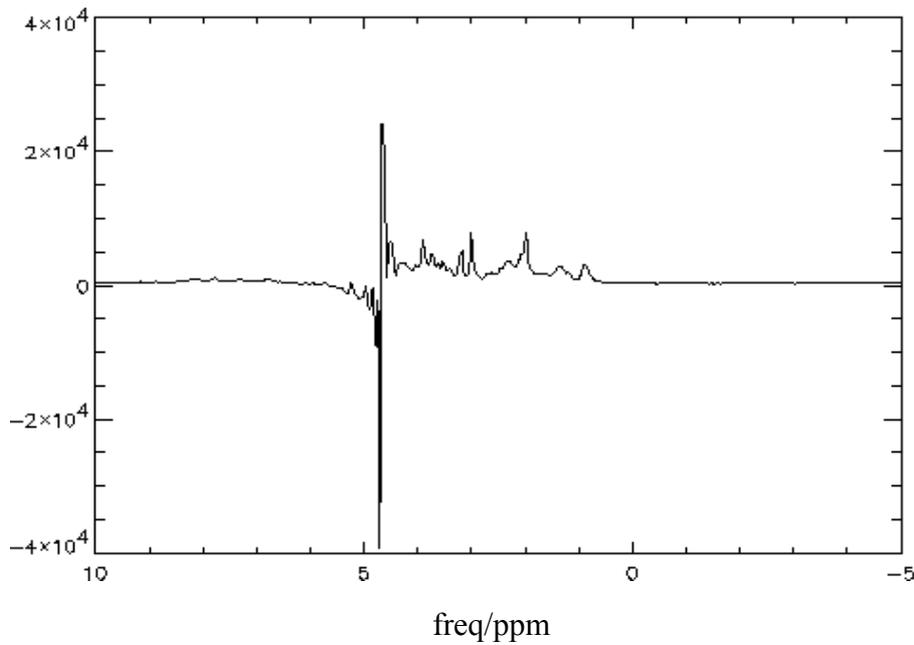
**Fig. 3.2-2** Spectrum of *in vivo* signal of rat brain acquired without WS after removal of water components. Water signal was extracted by MPM with 300 complex data points, reconstructed with 600 data points, and subtracted from the original signal. Large residue exists due to imperfect fitting of the last 300 points of water signal.
