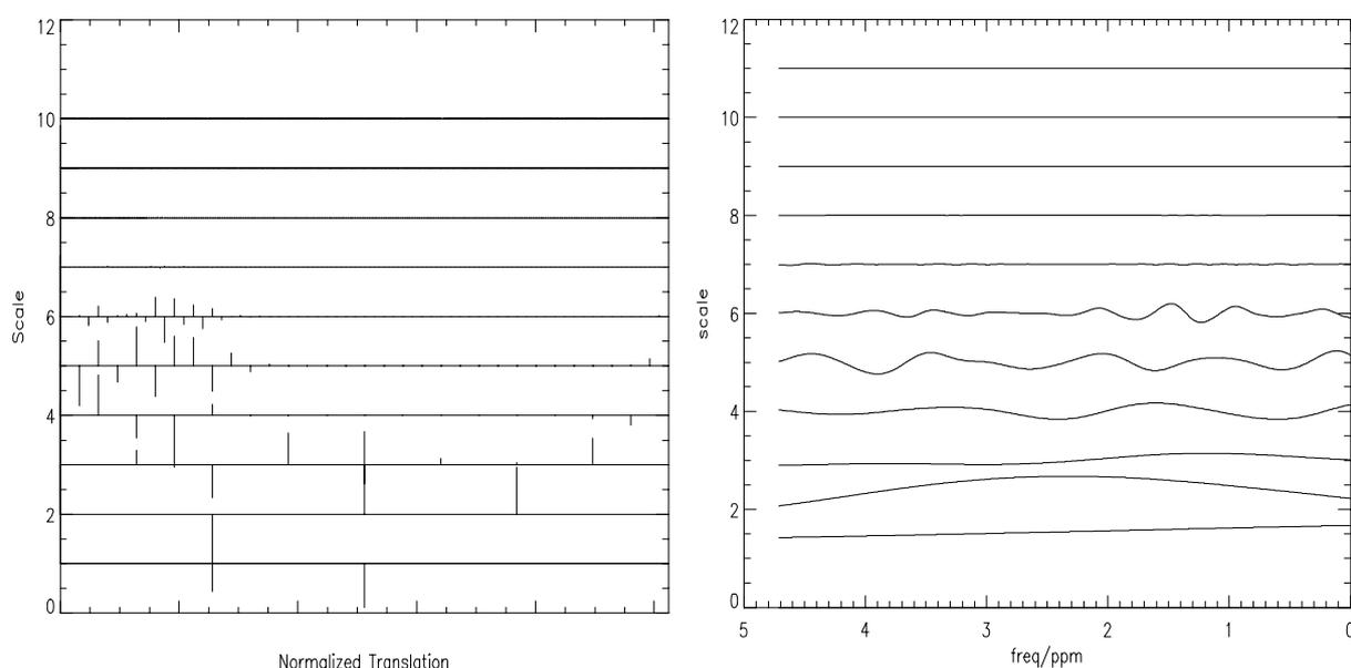
**Fig.3.6-5** Wavelet representation (a, left), of simulated baseline, and reconstructed baseline components (b, right) from wavelet coefficients of each scale. Note that the WTCs are shown for the whole spectrum of 20 ppm but the spectral components are shown only for the range of 0 ~ 5 ppm, corresponding to the first quarter of normalized translation in (a).
