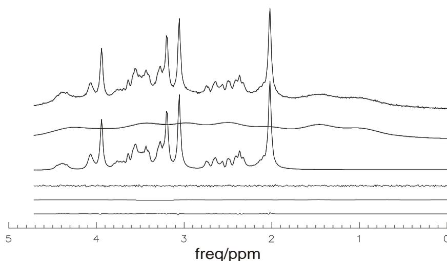
**Fig. 3.7-6** An example of spectral fitting with simulated signals from 6 metabolites and artificial baseline. Displayed from top to bottom are the test and the fitted spectra overlaid, the artificial baseline and fitted baseline overlaid, the simulated spectrum and the fitted overlaid, and the residues of total spectrum, baseline and metabolite spectrum.
