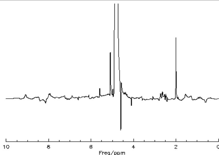
**Fig. 3.4-9** Water unsuppressed spectrum of NAA measured with spoiler gradients (PRESS, spoiler gradient strength = 67 mT/m).
