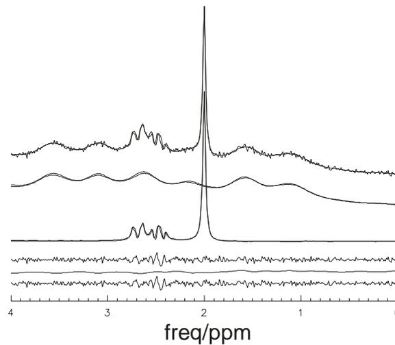
**Fig. 3.7-10** Fitting of a phantom spectrum with added artificial baseline. From top to bottom are the total test spectrum and the fitted spectrum, artificial baseline and fitted baseline, measured spectrum and fitted spectrum, all overlaid, and the residues of total spectrum, baseline and NAA spectrum.
