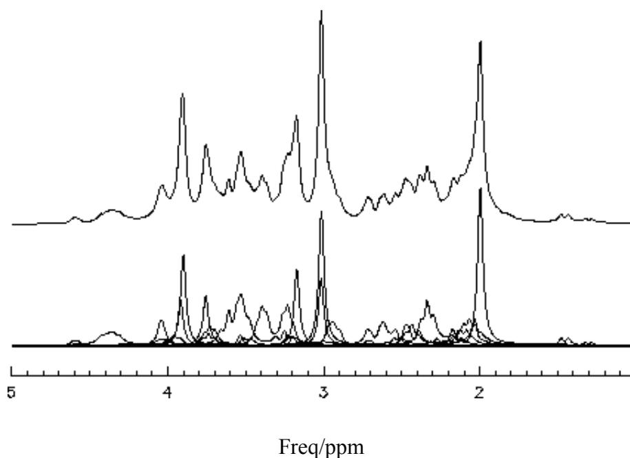
**Fig. 3.1-3** Simulated proton spectra of main metabolites in animal brain. The metabolites and the simulation parameters are the same as those in Fig.3-1. Lorentzian linebroadening of 8 Hz was applied on the simulated time domain signals to approximate the ideal *in vivo* spectra. The lower trace are the metabolite spectra overlaid. The upper trace is the sum spectrum of the metabolite spectra.
