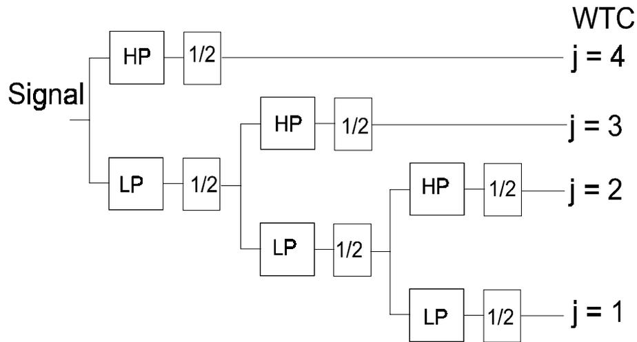
**Fig. 3.6-2** Schematic illustration of DWT algorithm. HP and LP stand for high pass and low pass filters, respectively; WTC stands for wavelet coefficients.
