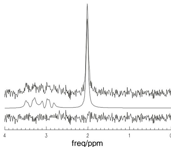
**Fig. 3.7-9** A representative spectral fitting of the MC study. From top to bottom are: the measured spectrum with added noise, the fitted spectrum and the residue.
