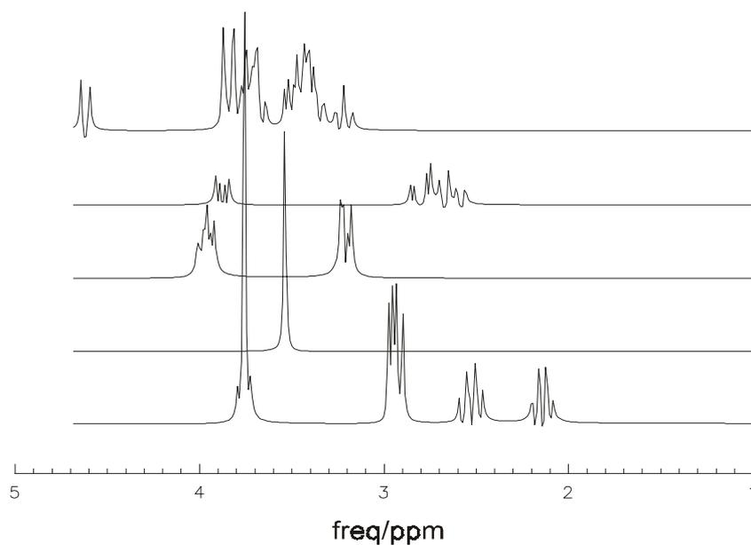
**Fig. 3.5-2c** Simulated spectra (from top to bottom): Glc, Asp, PE, Gly, GSH.
