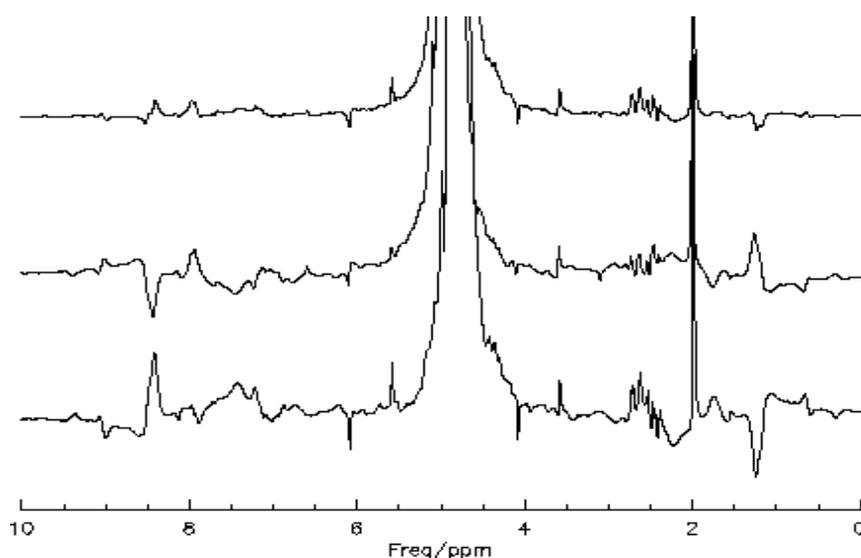
**Fig. 3.4-3** NAA spectra measured without water suppression and with positive gradient pulses (bottom), negative gradient pulses (middle). The upper spectrum is the combination of the two, scaled by a factor of 0.5. The experimental parameters are: PRESS, TE = 20 ms, Voxel size = 1 cm<sup>3</sup>, NA = 16. NAA concentration = 100 mM, spoiler gradient intensity = 67 mT/m.
