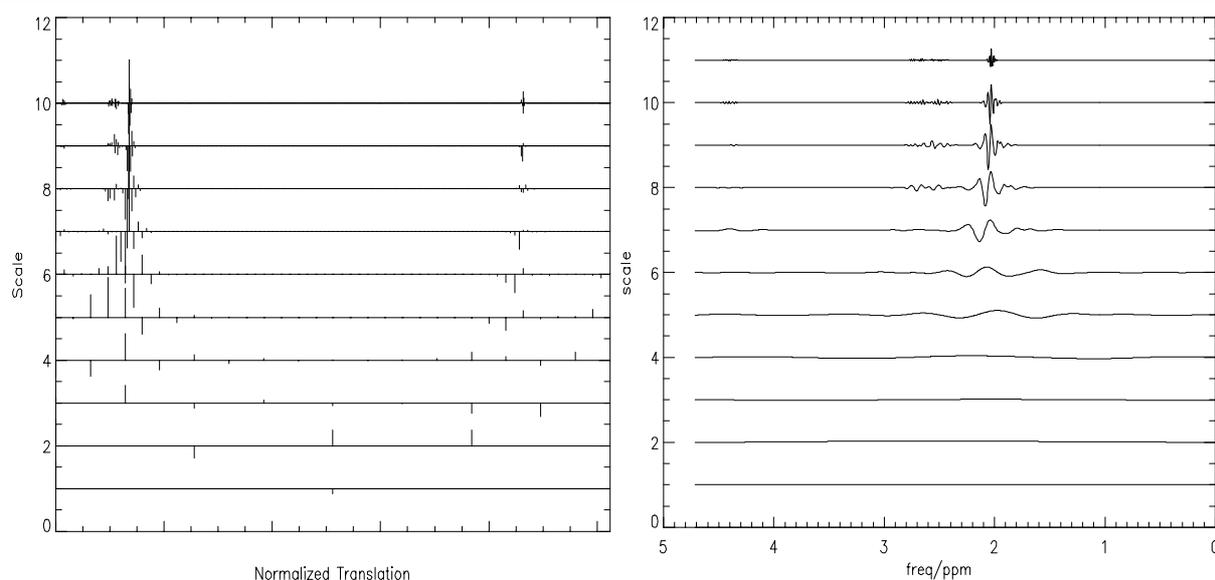
**Fig. 3.6-4** Wavelet representation (a, left), wavelet coefficients distribution on each scale of a simulated frequency domain NAA signal with linewidth of 3 Hz; Reconstructed NAA spectral components (b, right) from wavelet coefficients of each scale. Note that the WTCs are shown for the whole spectrum (20 ppm) while the spectral components are shown only for the range of 0 ~ 5 ppm, corresponding to about the first quarter of the normalized translation in (a).
