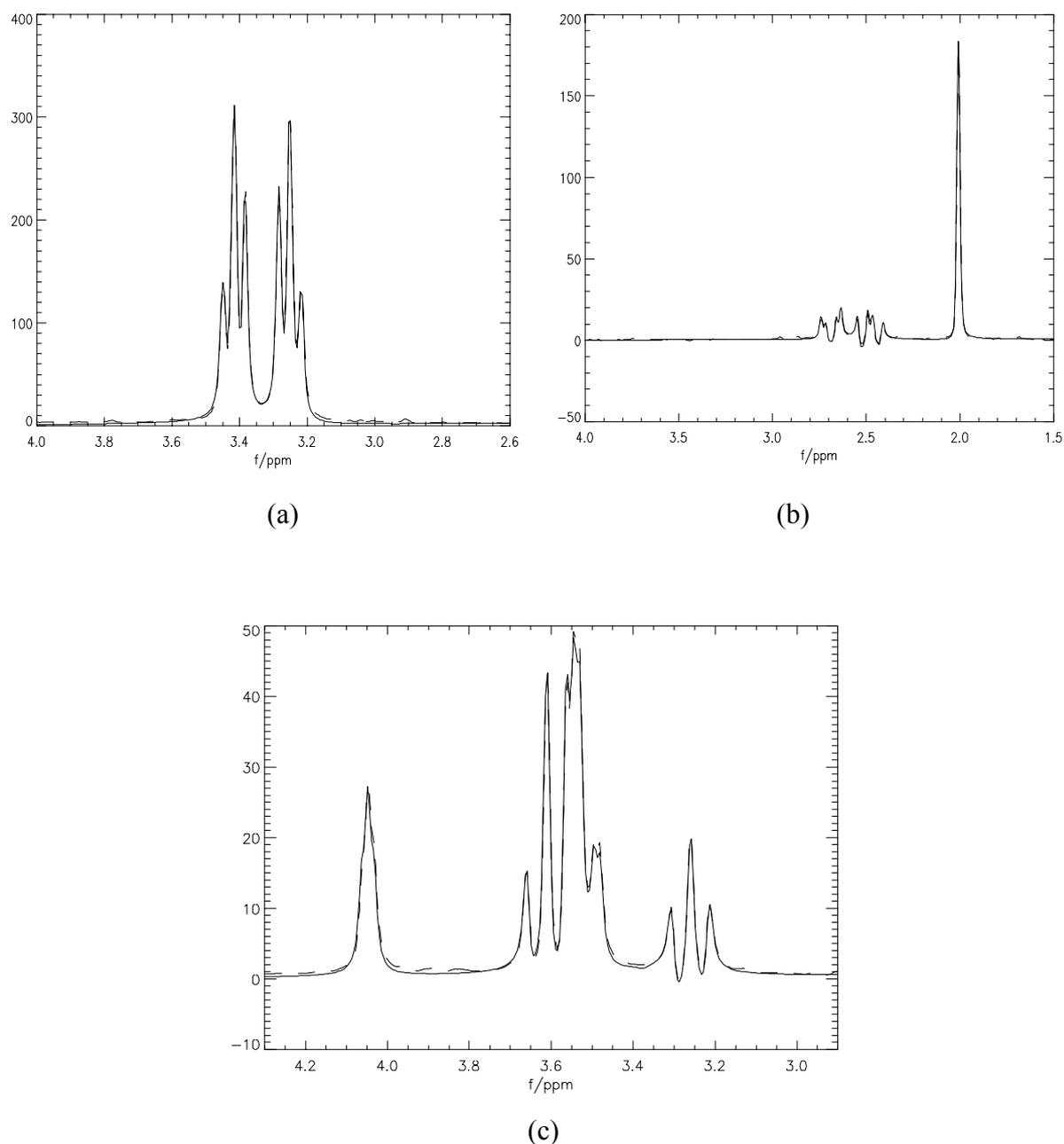
**Fig. 3.5-3** The measured phantom spectra overlaid with the simulated spectra of Tau (a), NAA (b) and Ins (c).
