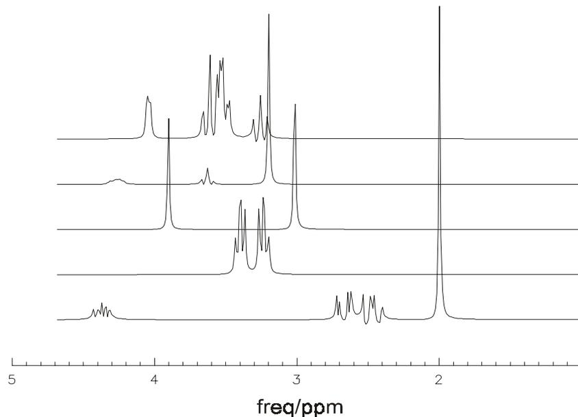
**Fig. 3.5-2a** Simulated spectra (from top to bottom): Ins, PCh, Cr, Tau and NAA.
