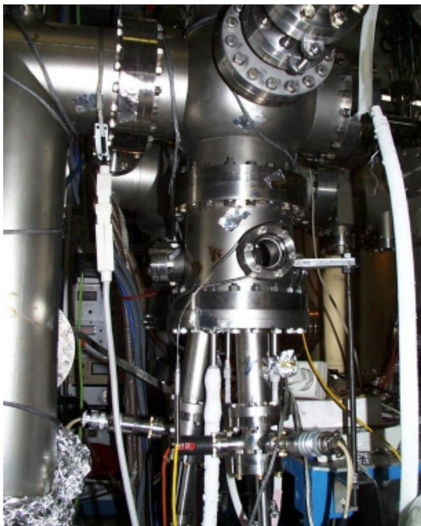
*FIG. 2 Our new metallization chamber.*
