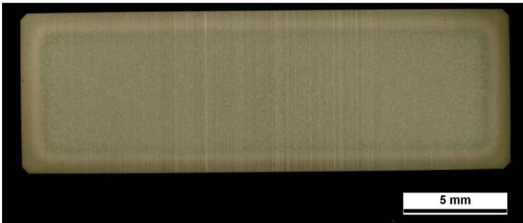
Figure 3.13 Sample sectioning for metallographic examination and hardness testing
