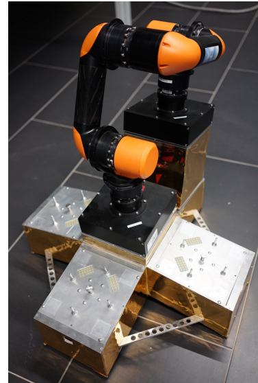
(b) The manipulator SIMA comprises two female interfaces for docking, here attached to a base camp. With connection to a power source, it can serve as agent with limited mobility, e.g., wander by attaching to male interfaces.
