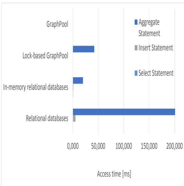
**3.20a:** Performance comparison of core & aggregate queries for multi access scenarios: overall, my [GraphPool](#) outperforms all competitors for all query types for multi-component access.
