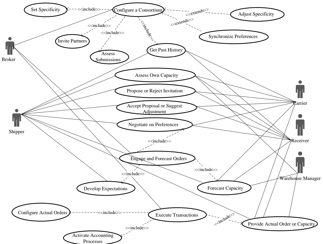
Figure 21: A use-case diagram to describe functional requirements
