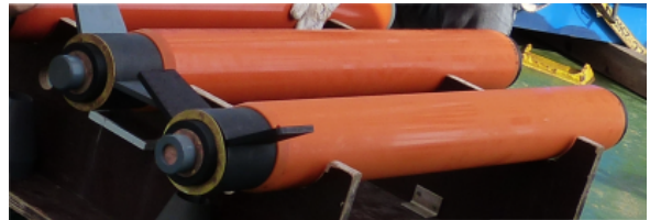
Figure 2.7: Two sensors of the Sea Spy gradient magnetometer system, prepared for operation during the cruise SO230.
