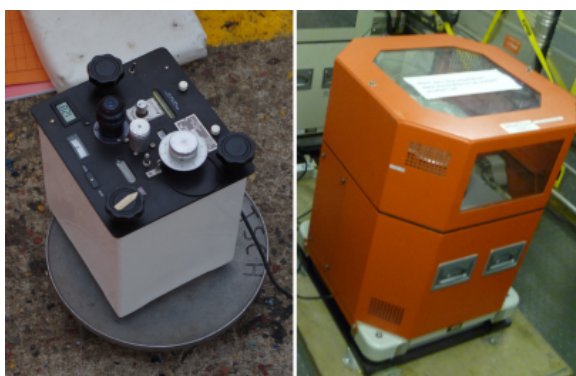
Figure 2.6: Gravimeters used during the cruise SO230. Left image shows the LaCoste & Romberg land gravimeter G480 for tie measurements in the harbour of Durban, RSA. Right image shows the Bodenseewerke marine gravimeter system KSS32M (S/N 22) in the gravimeter room of RV Sonne.
