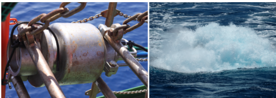
Figure 2.2: Air guns were used for the generation of the seismic signal. Left image shows a single air gun during the cruise SO230. Right image illustrates a shot (release of highly pressurized air into the water for generation of the seismic energy) as observed at the surface.
