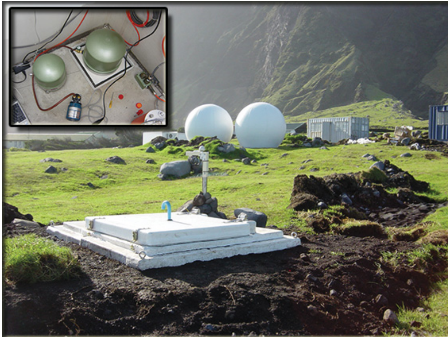
Figure 7: Permanent station TRIS located on TdC and equipped with an STS-2 (inset).
