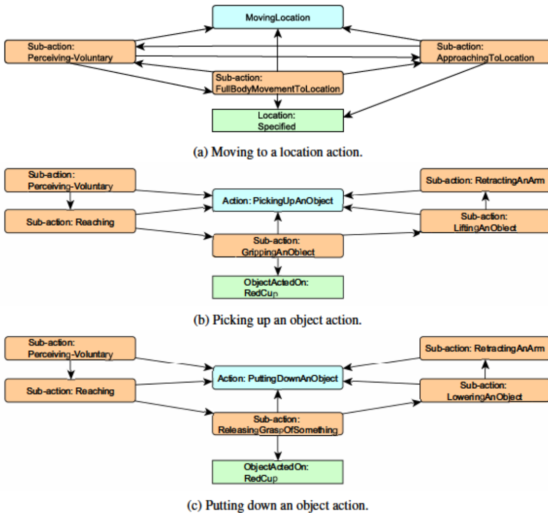
Figure B.2: Actions and sub-actions involved in the task of picking and placing a cup and bowl from the counter to the table.
